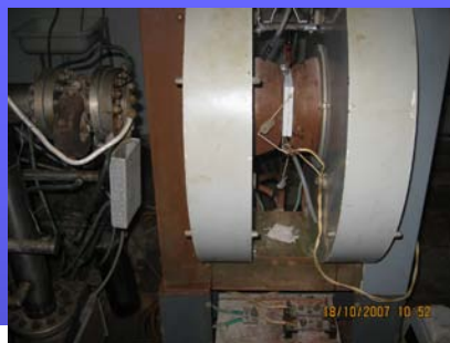
Thermomagnetic rig on the basis of electron accelerator LINAC-4
